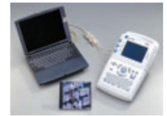
PC Direct Connectivity provides a direct connection to PC via serial port and cable
